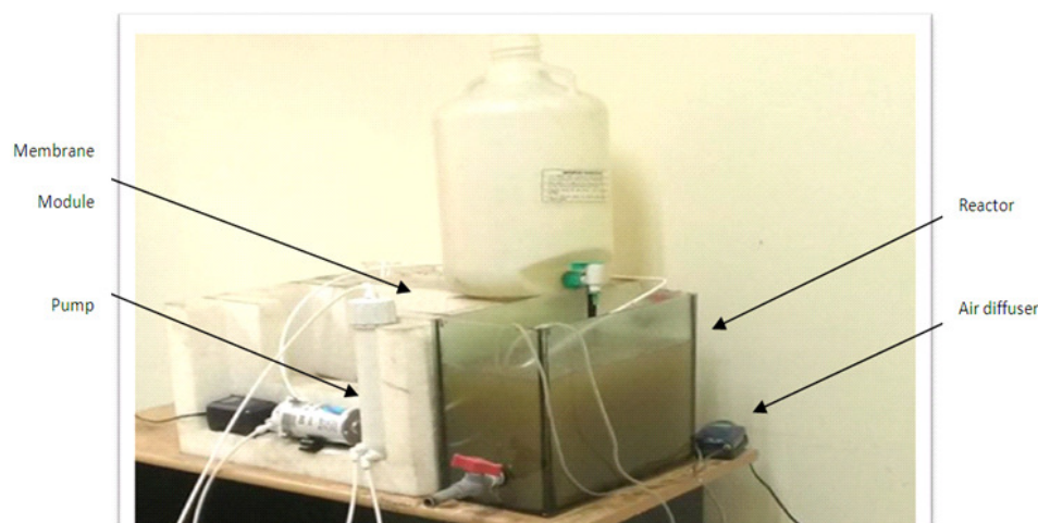
Fig. 1 : Experimental set up of Membrane Bioreactor used in present study.
