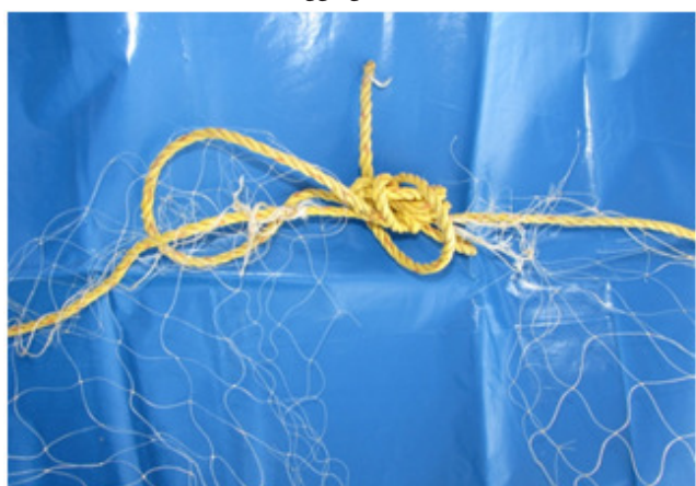
Joining of two unit at head rope
