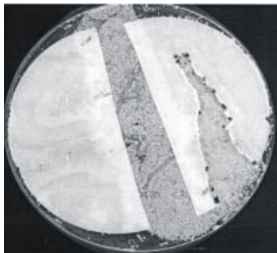
Fig. 6. Image from scanning a replicate in a choice test with untreated and 12 per cent 2-phenoxyethanol treated filter paper after 8 days exposure, showing that most termites (colony CR2) were attracted to treated filter paper and food consumption on the untreated filter paper was negligible.
